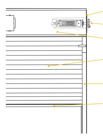
**BRACKETS** - Steel with powder coated finish to match curtain. Bolt to guide assembly and support counter-balance shaft and curtain.
